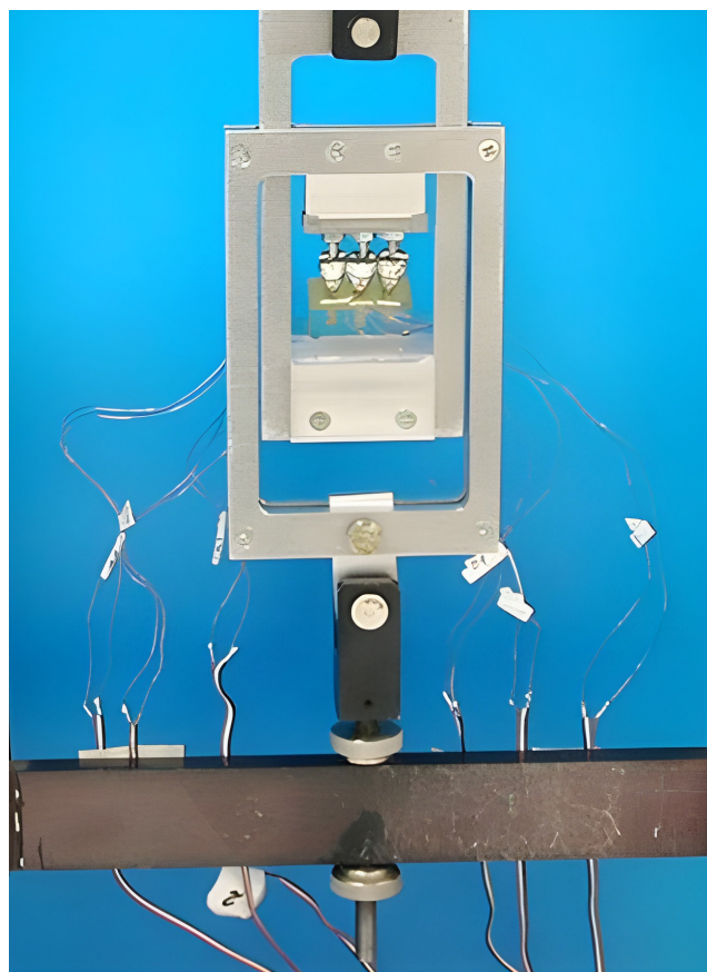
Fig. 3. Loading device with the test model
