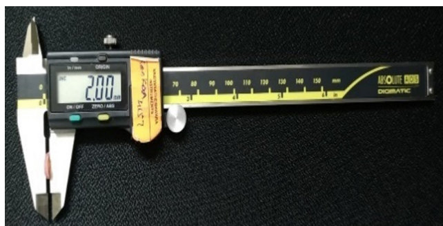
Fig. 1. Prepared root sections were measured using a digital caliper prior to push-out bond strength (POBS) testing to standardize the sample thickness, and only samples measuring 2 mm in thickness were included
