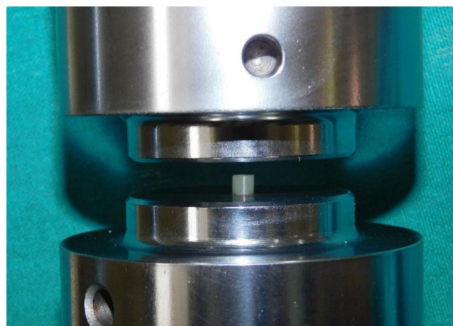
Fig. 1. Sample placed in a universal testing machine (Model No. 8801; Instron, Norwood, USA)
