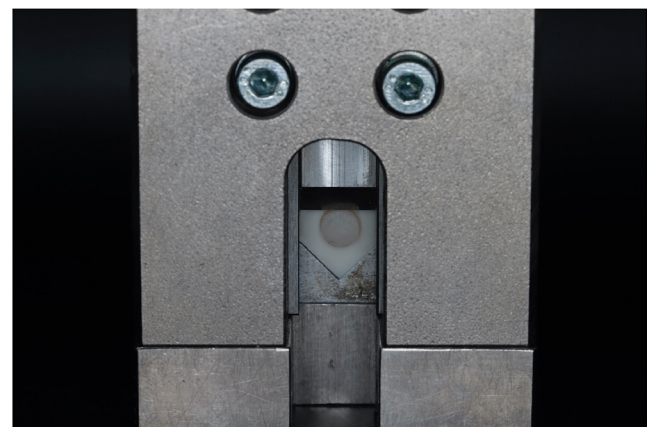
Fig. 3. Shear bond strength (SBS) testing setup using a universal testing machine (zwickiLine Z0.5 TN; ZwickRoell, Ulm, Germany) with a bonded ceramic–composite specimen
