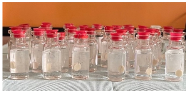
Fig. 2. Glass jars containing the ion release test samples
